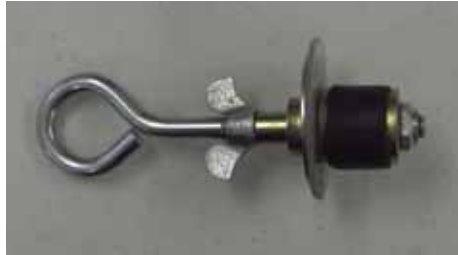
Figure 6.6 – pump disassembly tool F-00097
