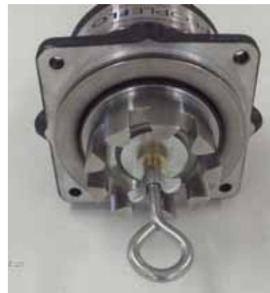
Figure 6.31 – rotor assembly in place
