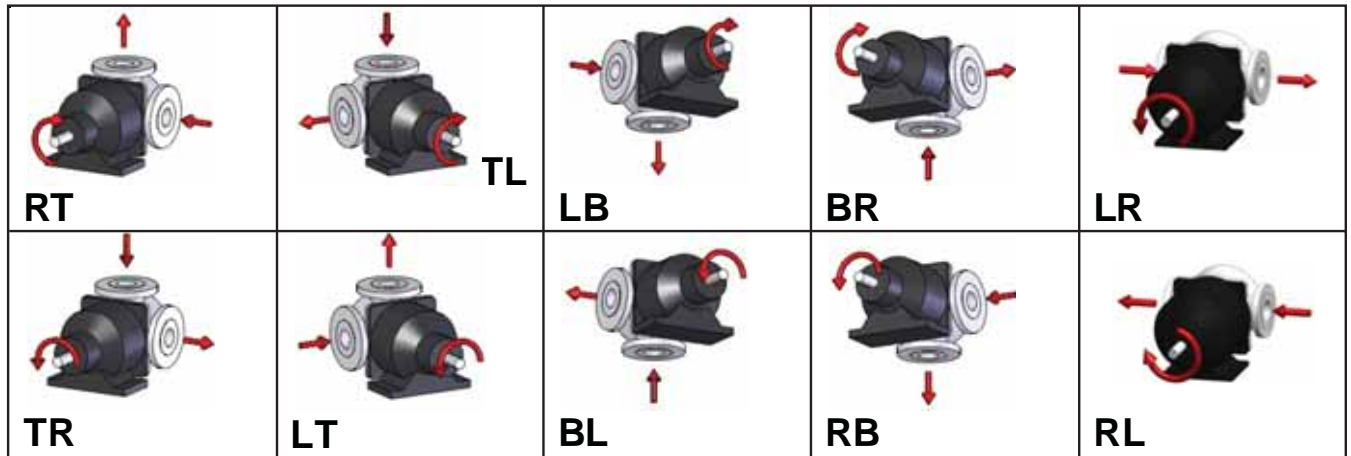
Figure 3.1 – eight possible port orientations
